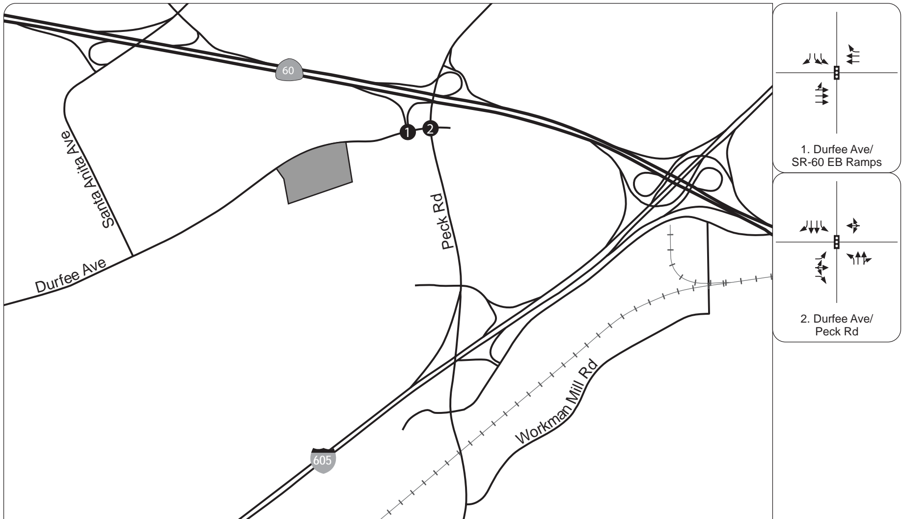
Figure 3.7-1 Location of Study Intersections and Existing Lane Configuration
